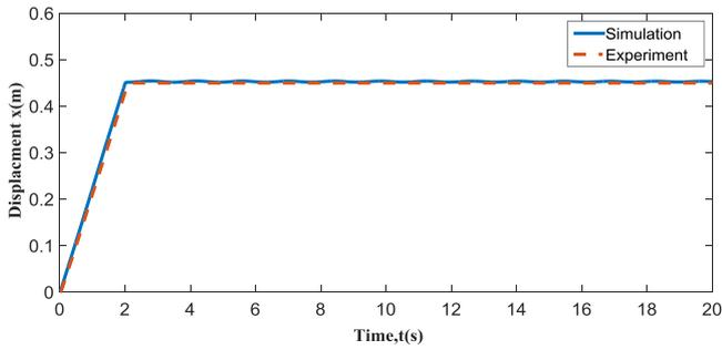
Figure 7. Cart displacement for both simulation and experiment
