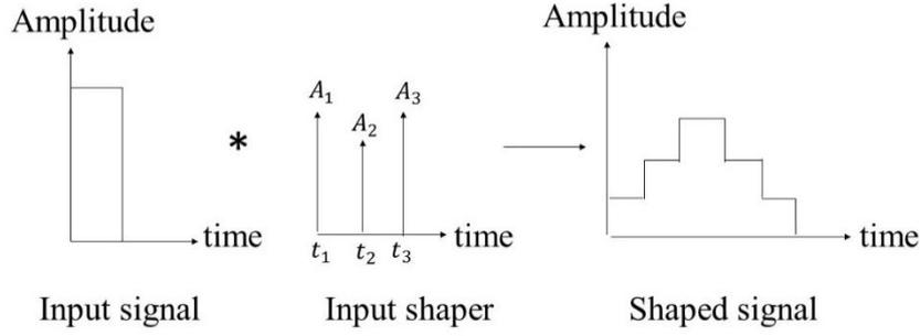
Figure 6. Process of input shaping
