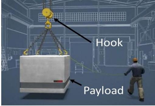
Figure 1. A double-pendulum overhead crane system
