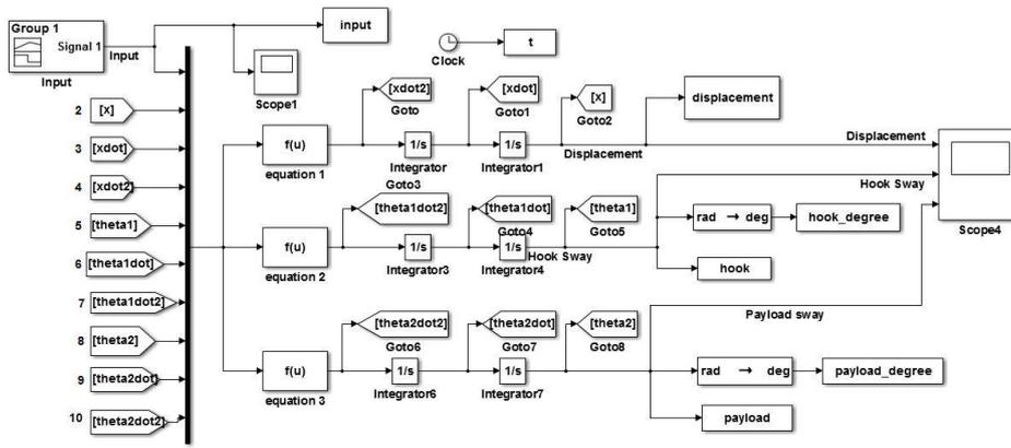
Figure 3. Simulink block diagram for the double-pendulum overhead crane system
