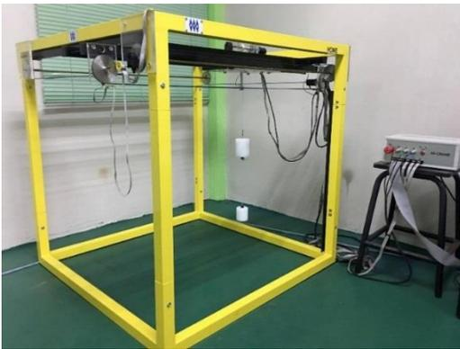
Figure 4. Experimental setup of a double-pendulum overhead crane system
