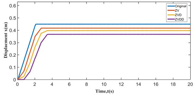
Figure 12. Cart displacement for the experimental double-pendulum overhead crane
