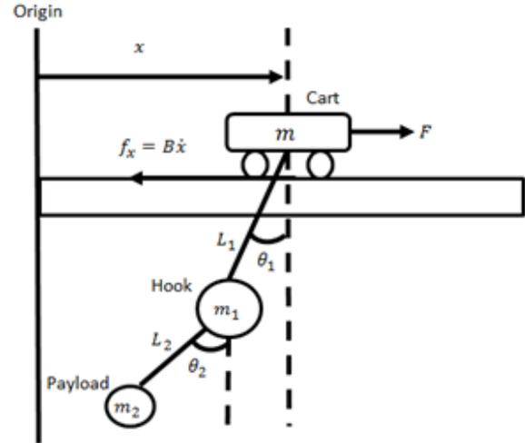
Figure 2. Schematic diagram of a double-pendulum overhead crane system
