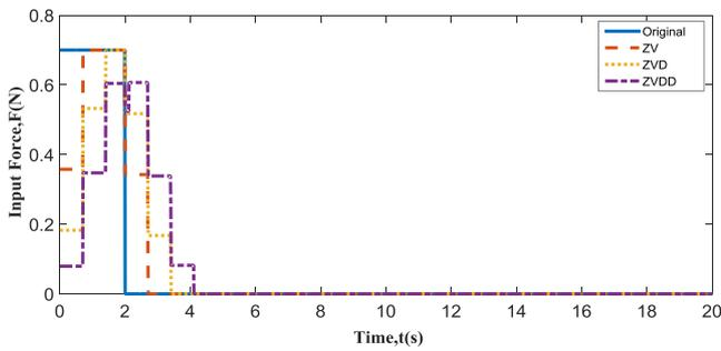
Figure 11. Input signal after the implementation of input shaper
