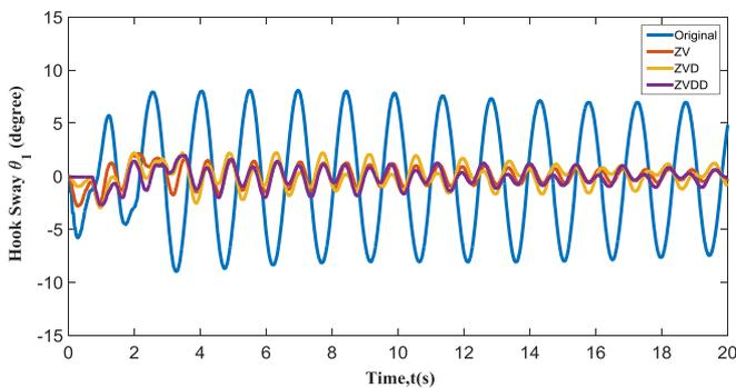
Figure 13. Hook sway for the experimental double-pendulum overhead crane system
