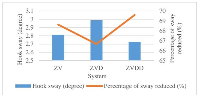
Figure 14. Performance of ZV, ZVD and ZVDD shaper on sway control
